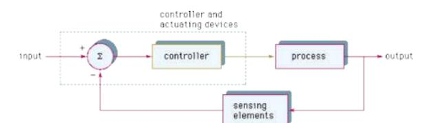
The input to the system is the reference value, or set point, for the
